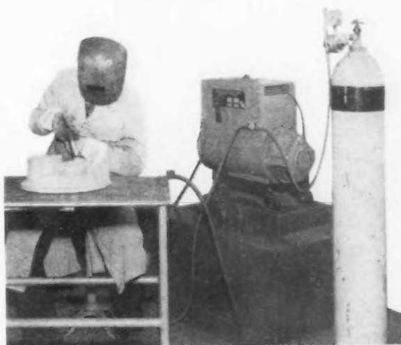
FIG. 1 —Setup for Inert-Arc welding includes a standard air-cooled electrode holder, a dc arc-welder, and a bottle of helium with regulator, gas flowmeter and hose.
